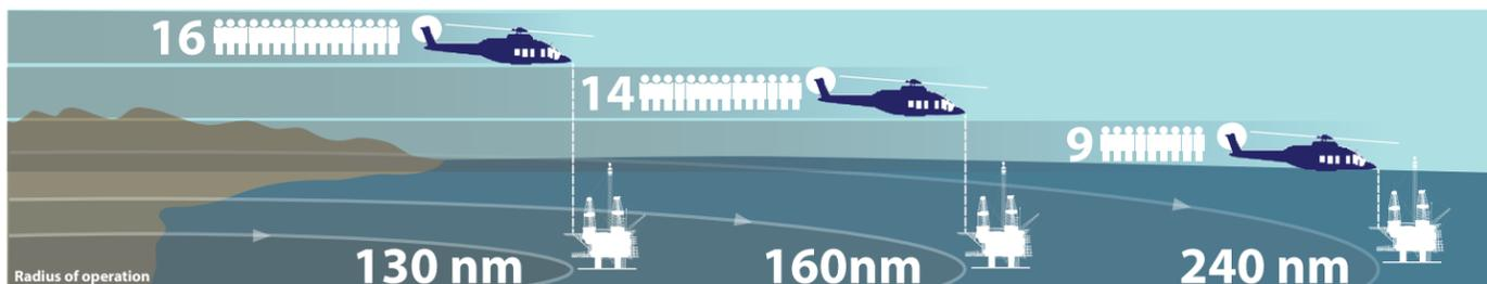
Radius of operation Max GW, 6Kft ISA+20, OGP configuration, standard tank, CAT A w/JAROPS fuel reserves, 255lb pax wt
